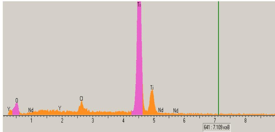
Fig. 1. EDS spectroscopy of  $TiO_2/Nd$  samples with  $Y^{3+}$  on the surface
